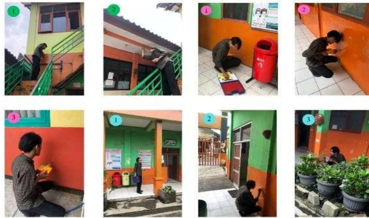
Figure 7. The Hammer Test Process at SDN 1 Jambudipa (Source: Personal Documentation, 2025).
