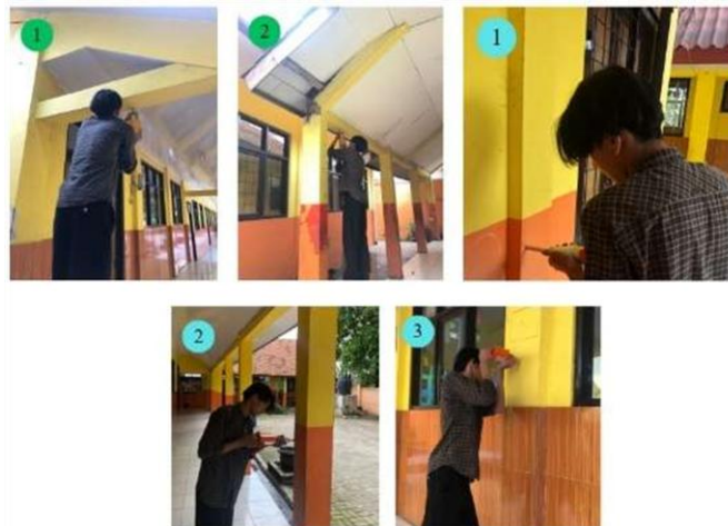
Figure 8. The Hammer Test Process at SDN 2 Jambudipa (Source: Personal Documentation, 2025).
