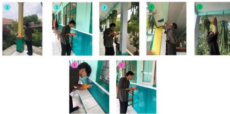
Figure 10. The Hammer Test Process at SDN Gandrung Endah (Source: Personal Documentation, 2025).
