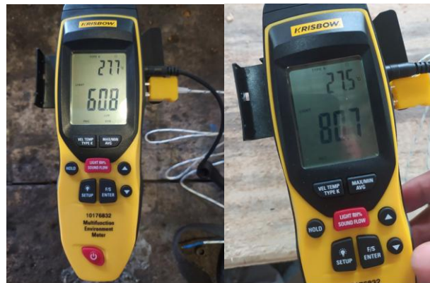
Figure 2. Documentation of Light Intensity Measurement in the Work Area and Under Light Source: AAP Putra, (2025).
